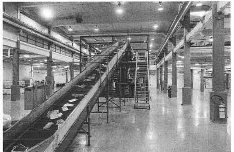
A conveyor belt carries batteries to be recycled into reusable material at Li-Cycle. Libby March for The New York Times
